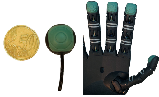
Fig. 9: Left: the SINGLEX stand-alone tactile pressure sensor version. Right: FTS tactile pressure sensor mounted on a robot finger. Images used with permission from Seed Robotics ( https://www.seedrobotics.com/ ).
