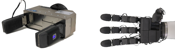
Fig. 10: Left: a flat version inspired by Tomo et al. (2018a). Right: a multi-curved version inspired by Tomo et al. (2018b). Images with permission from Xela Robotics ( https://xelarobotics.com/ ).
