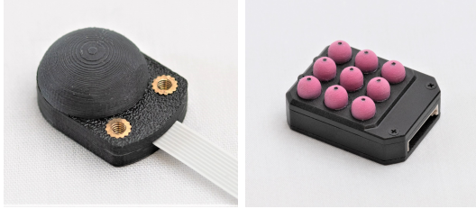
Fig. 11: Left: Single 3D force tactile sensor. Right: A slim tactile sensor array (PapillArray Sensor) available in different configurations. Images from Contactile ( https://contactile.com/ ), licensed under CC BY-NC-ND 4.0.
