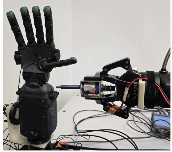
Fig. 1 Setup of the impulse response localization task. The UR5e robotic arm is shown applying controlled pokes to the hand using a solenoid actuator with a metal indenter.
