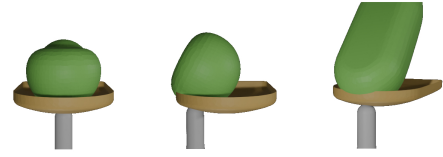
Fig. 3. Transferred BioTac sensor (green) to align it with the DIGIT sensor surface (gold), in order to collect paired 3D deformation meshes.
