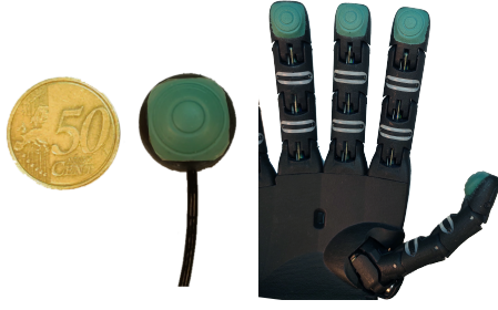
(a) Left: the SINGLEX stand-alone tactile pressure sensor version. Right: FTS tactile pressure sensor mounted on a robot finger. Images used with permission from Seed Robotics ( https://www.seedrobotics.com/ ).
