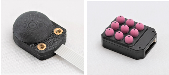
(c) Left: Single 3D force tactile sensor. Right: A slim tactile sensor array (PapillArray Sensor) available in different configurations. Images from Contactile ( https://contactile.com/ ), licensed under CC BY-NC-ND 4.0.
